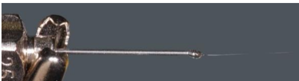
Fig 2: jet coming out from the tip of the spinneret
